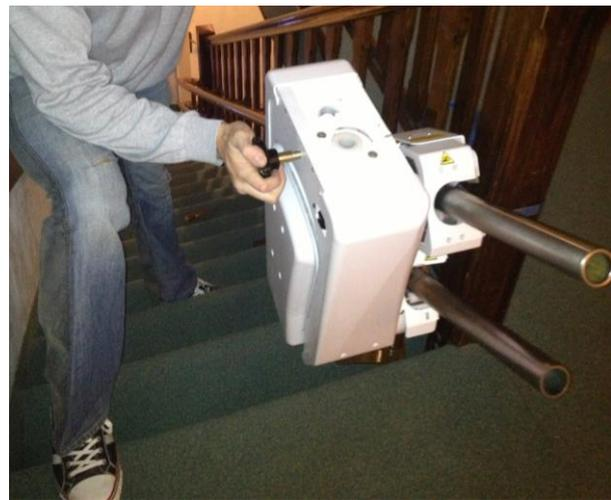
**Step 3:** Take of the side and front plastic covers. Then put the chair into the fixation and fix and lock it with the screw and washer from inside the drive unit.
