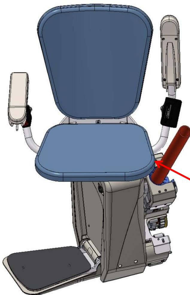
The seat cannot rotate more because of clashing with the rail tube
