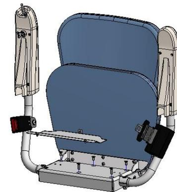
Upper part of the chair is mounted onto „U“ console of the drive unit with screws M6.
