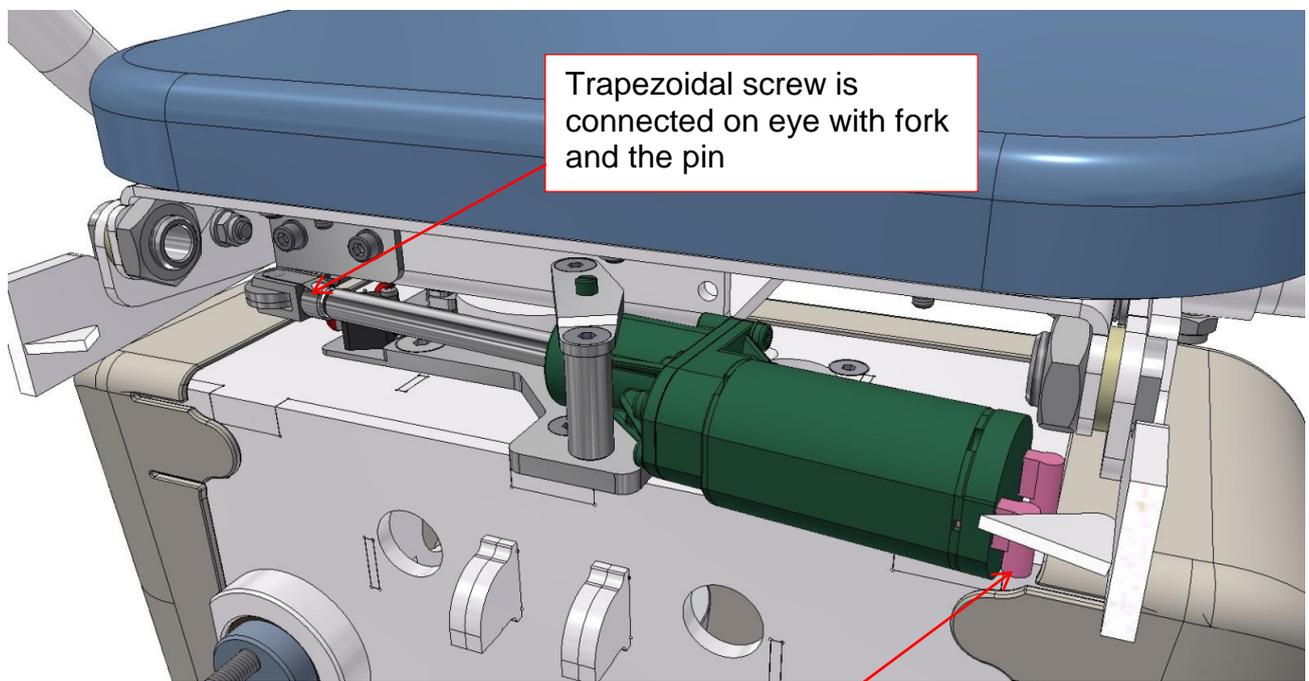
Trapezoidal screw is connected on eye with fork and the pin
