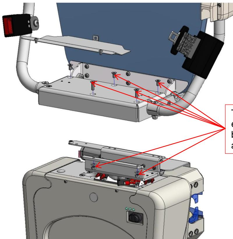
Two screws on front side are ensured with nuts from the bottom. Two screws on rear side are without nuts.
