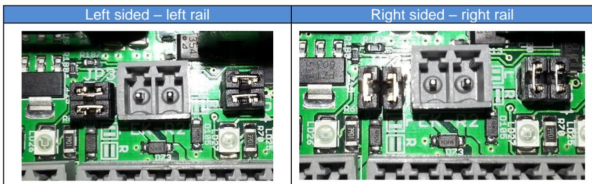
**CAUTION: Proper jumper setting is absolutely necessary for the correct and safe function – safety elements in the drive direction.**
