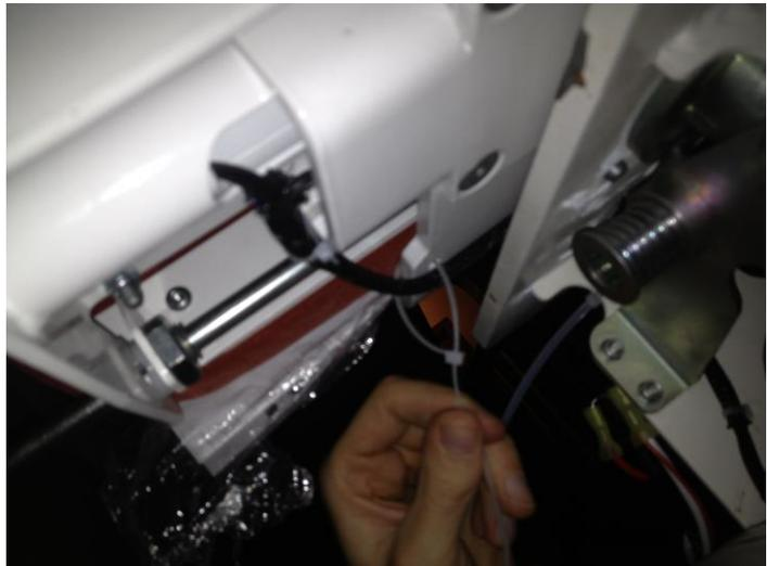
**Step 5:** Now drive the unit down and up to check if the seat passes all steps and if the clearance is ok.
