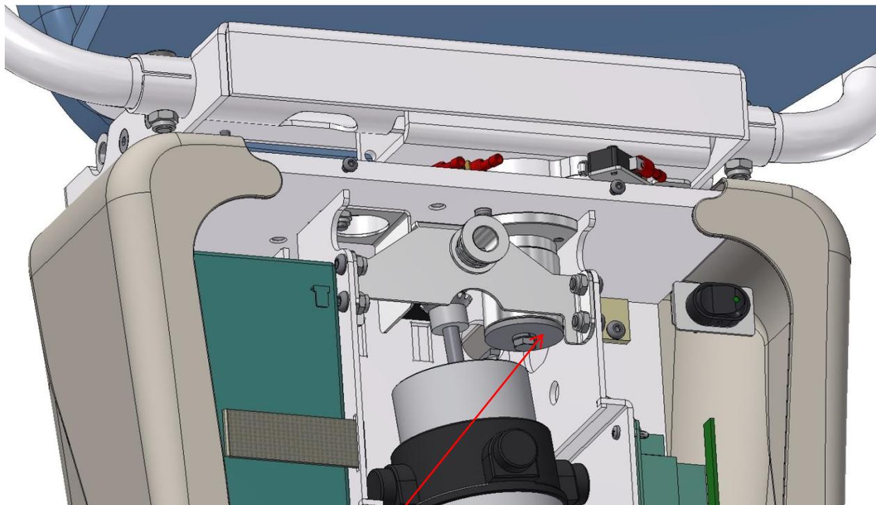
The big washer, spring washer and screw M6x20, DIN 933 are inserted in production factory. It protect the seat for upward movement and disconnection. It is important for good function of the automatic swivel.
