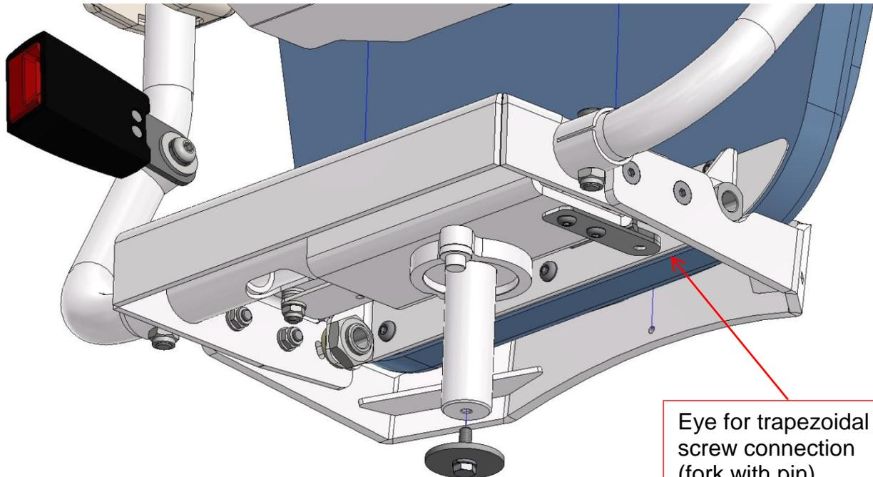
Eye for trapezoidal screw connection (fork with pin)
