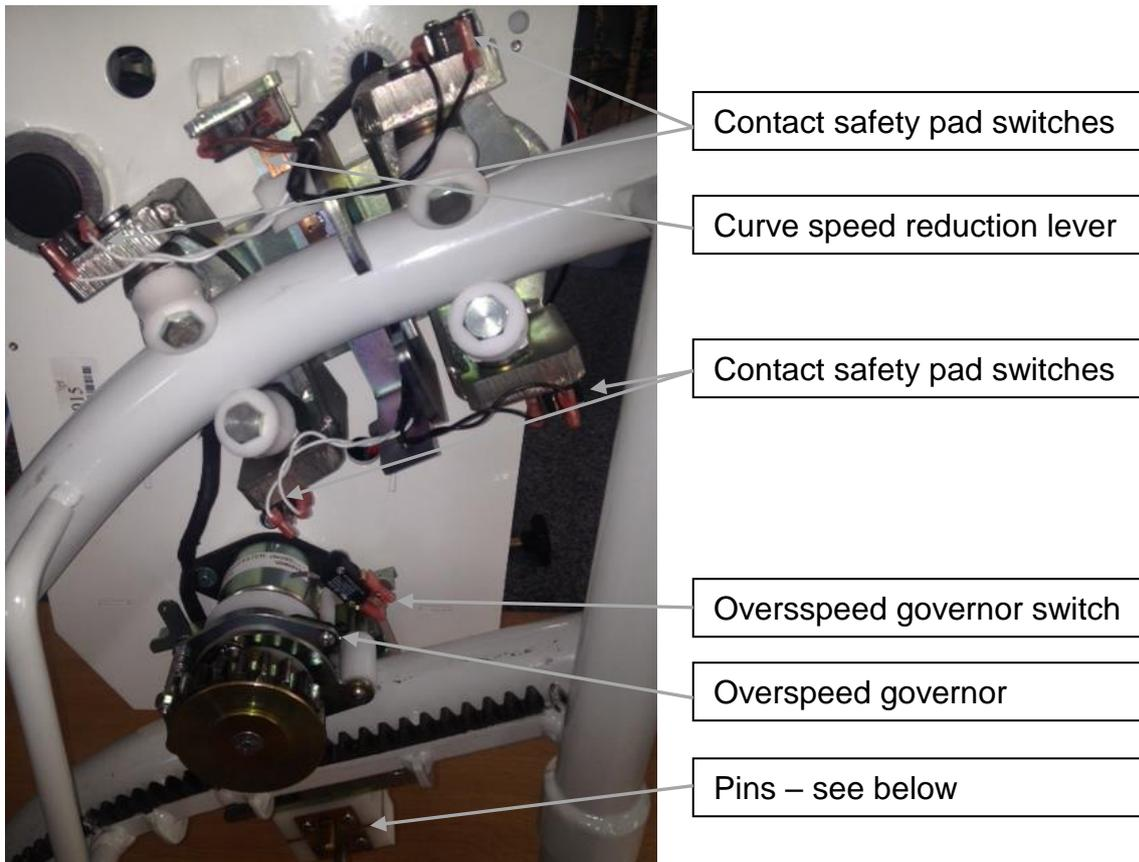
The lower pin is the ultimate stop pin. This activates the safety switch at the end of the rail (in case the normal stop would not work). The upper pin is responsible for taking the positive charging current and at the same time activates a slow down switch when at hitting the landing station charging cams. On an intermediate stop assembly this pin is pressed further inside and then additionally activates the intermediate stop switch. This only happens on intermediate stops, not on end stops.
