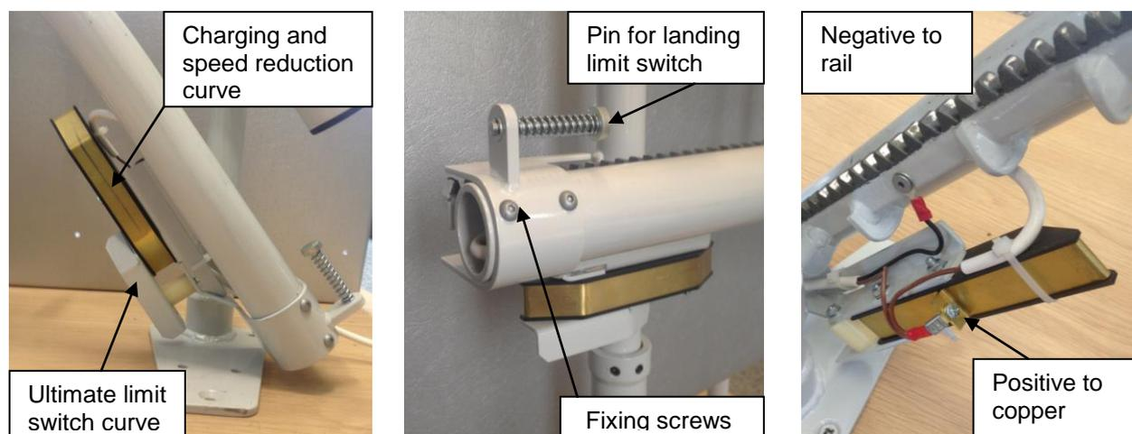
On inclined rail parts the electrical ground is transferred to the board via the rack. But in horizontal section this ground connection can be unstable. Therefore, in case of a horizontal stop or an intermediate landing it is necessary to add a copper plate onto the upper tube. This copper plate ensures the electrical ground connection to the stairlift board.
