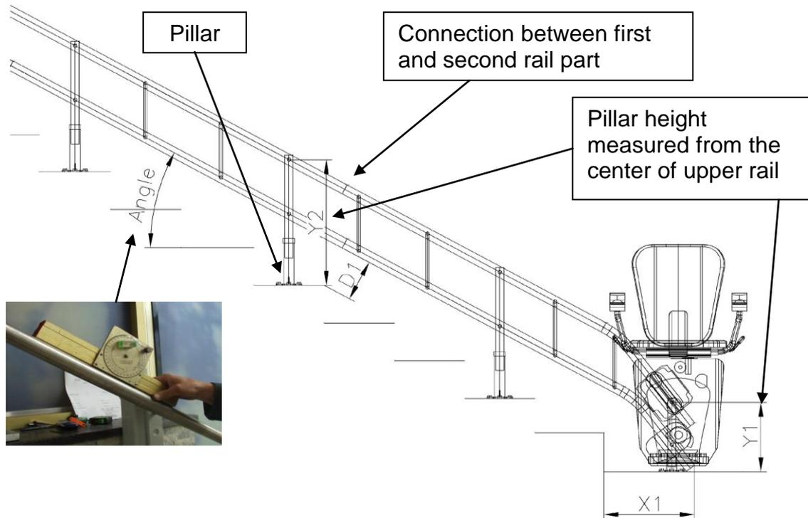
**Step 1: Start fixing the rail from the bottom! Do not start installation from the top.**
