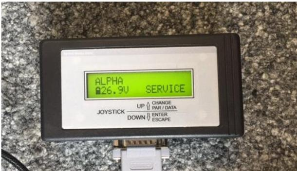
**WARNING:** After installation and setting of all the parameters, set the switch S2 back to user's mode. Otherwise, after the chair stairlift reaches the final station the entrance into the menu can be blocked – and whole control system can be blocked as well.
