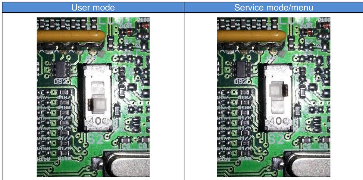
**WARNING: After the platform installation and setting all service menu parameters, push the switch S2 to the position for user menu!!!**
