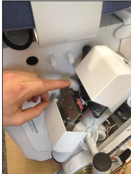
The lever is activated by the rail. When the lift drives into a curve the rail bend presses the lever so that it activates the speed reduction switch. If the unit does not slow down correctly please bend the lever a little so that the speed reduction switch is pressed even more when the lift drives into a curve. Make sure you do not bend it so much that it drives slow also on straight sections.
