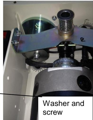
**Step 4:** Use cable ties to fix the connection cable between from the chair to the drive unit. Makes sure the seat can freely rotate with the cable getting twisted or squeezed. Before fixing the cables rotate the seat to the maximum, then fix cables in place and rotate back and forth to see if the cable moves freely.
